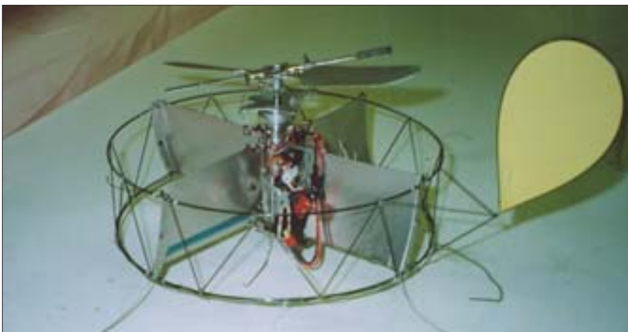
Mara Tishchenko's miniature helicopter will serve as the baseline for the university's MAV work.
