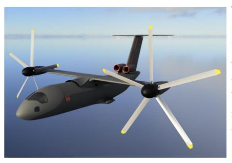
The AGRC-developed Arion is also endowed with unprecedented speed and embodies the immortal dream of VTOL – helicopter like hover and jet like cruise. Arion is a 48,000 lb **mixed power tiltrotor**, capable of delivering 5000 lb of cargo, or 20 fully
