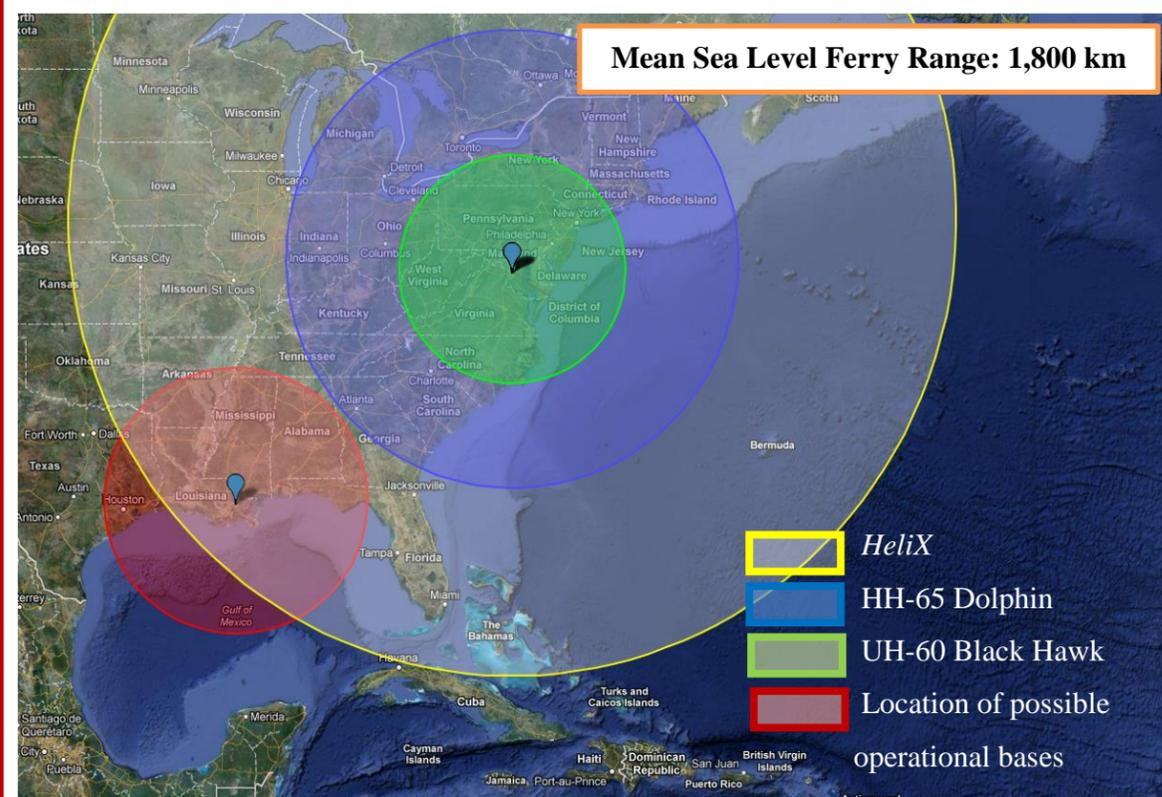
**LEFT:** The red circle seen in the figure to the left has a radius of 600 km centered on New Orleans, LA and the circumference indicates all the possible locations the operational base could be located. If **deployed from the US Coast Guard Surface Forces Logistics center**, in Baltimore, MD, the *HeliX* clearly outperforms both the Dolphin and the Black Hawk, and is the only vehicle capable of reaching base camp without refueling.
