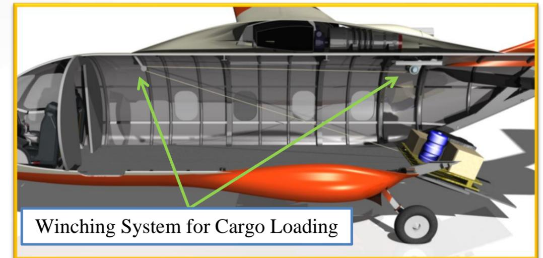
Winching System for Cargo Loading
